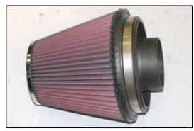
22. Install the provided adapter into the K&N® air filter and secure with provided hose clamp as shown.
