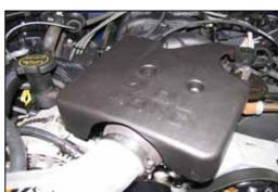
25. Reinstall the engine cover and secure with the factory mounting bolts.
