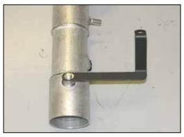
13. Install the provided tube mounting bracket (010081) onto the K&N<sup>®</sup> intake tube with the provided hardware as shown.
