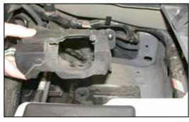
8. Pull firmly on the air inlet duct to dislodge it from core support and remove from the vehicle.
