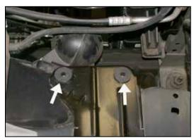
18. Install the two provided threaded inserts into the lower air box mounting plate at shown.
