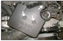
3. Remove the three engine cover mounting bolts shown.
