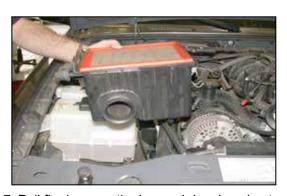
7. Pull firmly up on the lower air box housing to dislodge from the mounting grommets and remove lower air box from the vehicle.
