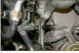
5. Depress the green locking tab and disconnect the crank case vent line from the valve cover as shown.
