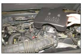
4. Remove the engine cover from the engine.
