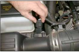
2. Disconnect the mass air sensor electrical connection and separate the harness from the stock intake tube wiring harness clip.
