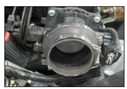
10. Install the silicone hose (084034) onto the throttle body and secure with the provided hose clamp as shown.
