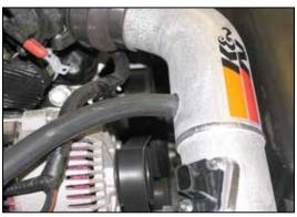
20. Install the provided crank case vent hose onto the fitting at the valve cover then attach the other end to the port on the K&N® intake tube.
