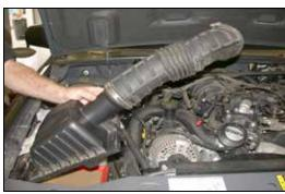
6. Loosen the hose clamp which secures the intake tube to the throttle body, release the two clam shell clamps which secure the upper air box lid and then remove the air box lid and intake tube from the vehicle.
