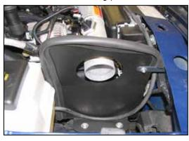
19. Install the heat shield assembly into the vehicle so the bracket lines up with the factory hole in the core support and the holes in the heat shield line up to the inserts installed in step #18. Secure the heat shield with the provided hardware.
