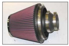
23. Install the provided silicone hose (084093) onto the air filter assembly and secure with the provided hose clamp as shown.
