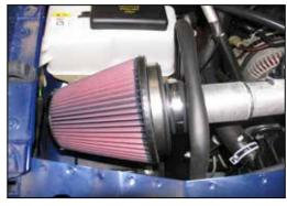
24. Install the air filter and secure with hose clamp provided.
