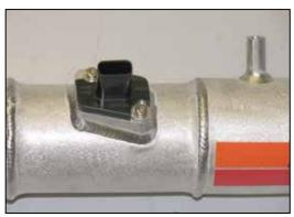
12. Using the provided mounting screws, install the mass air sensor into the intake tube as shown.
