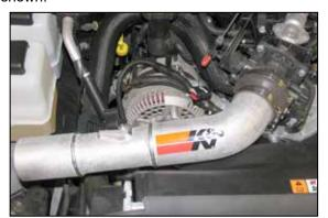
15. Install the K&N<sup>®</sup> intake tube into the throttle body and secure the bracket in place on the alternator with the bolt removed in step #14.
